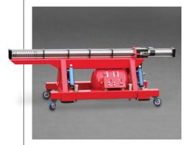
Moog Engineering provides shock testing services with a test system that is ideally suited for quick turnaround while minimizing over-testing. The system uses high energy mechanical impacts to replicate pyrotechnic events. Typical test articles are flight hardware and avionics. SRS levels can usually be replicated within a short lead time, and levels in excess of 40,000 Gs are generally easy to obtain on test articles weighing less
